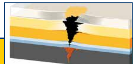
The consequence: Rust starts to form under the paint coat.
