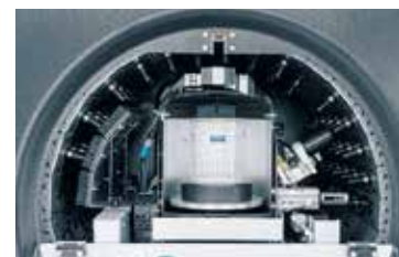
High-tech in the mixing room: the Daisy Wheel dosing system.
